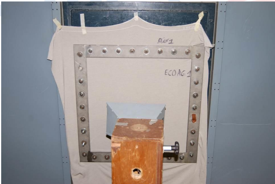
Picture 3: Test set-up with Horn antenna (1 - 6 GHz)
