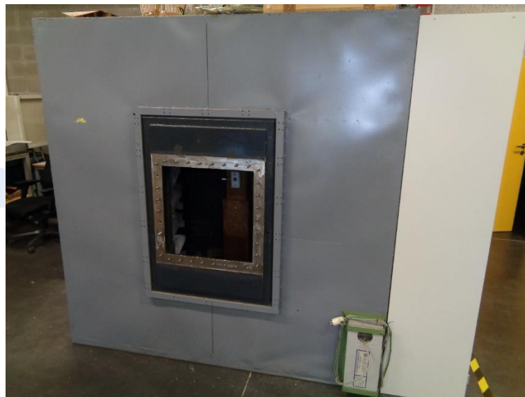
Picture 1: Picture of the IEEE Std 299 modified setup for the characterisation of the shielding effectiveness (SE) of materials
