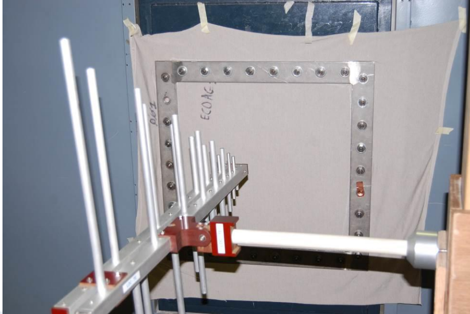
Picture 2: Test set-up with Log. Per. antenna (200 - 1000 MHz)
